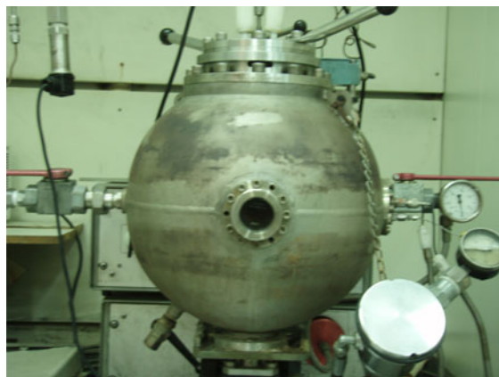
Fig. 1 Twenty liter spherical explosion vessel (20-L-Apparatus) for this study
